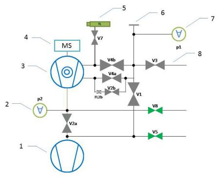
Fig. 11: The most important components of the vacuum diagram in PHOENIX devices
