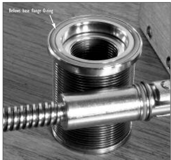
Bellows removed and bellows base flange O-ring exposed
