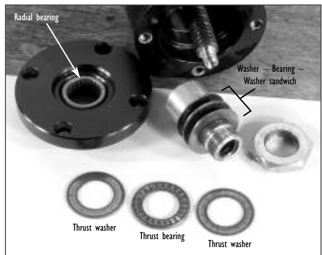
Drive nut and bearing block assembly parts
