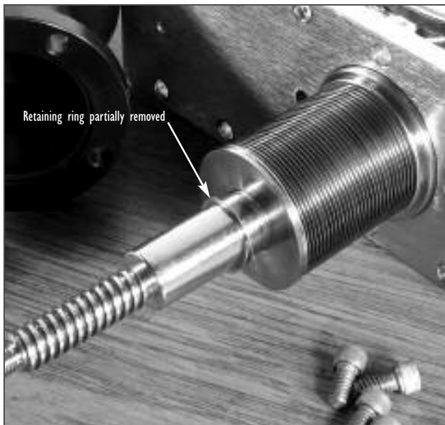
Remove the bellows retaining ring. Discard the retaining ring if a replacement is available.
