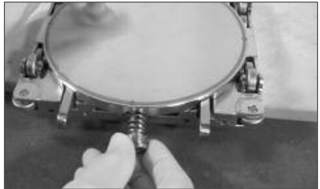
Install the gate spring
