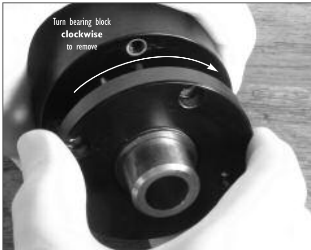
ACME thread on actuator stem is left-handed
