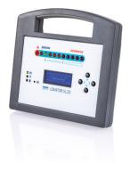
Mobile, industrial leak detector. The high flexibility of the LOKATOR VL20 allows for use with different refrigerants and for  $\rm H_2$  tracer gas with the same probe. The unit is the perfect tool for quick and accurate leak location whatever the gas to be detected.
