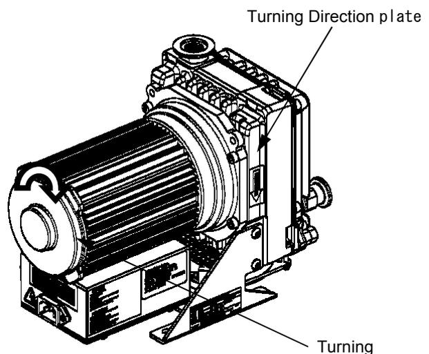
If you fit pump to vacuum system and control operation of vacuum pump by remote control, **first check pump itself for turning direction** and then fit it to vacuum system.
